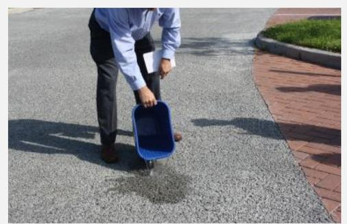
*Permeable, or porous, pavement allows water to seep into the ground instead of flowing over the land as part of stormwater.*
